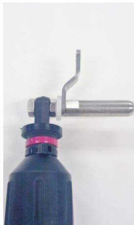
**Step 3** Hold the lever arm handle with a 7/16" wrench and the 5/16" hex bolt with a 1/2" wrench and tighten well. Note: Insure that the actuator can rotate freely, but remains snug.
