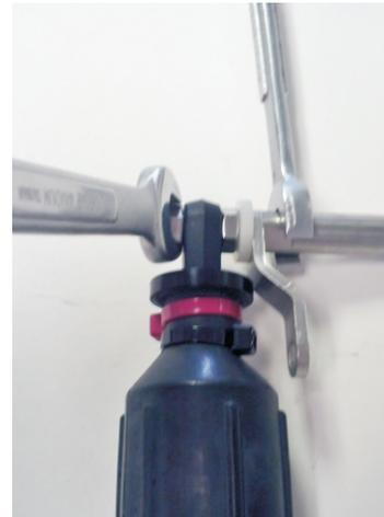
**Step 4** Attach the lever arm to the PR500 Bracket using the 5/16" phillips head machine screw and self locking nut. Use the white nylon washers on each side of the bracket. Tighten securely, but not too much. The handle should rotate with minimal force.
